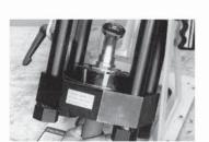
3. Loosen knob and tilt press as necessary. Insert hose assembly from below the base plate and between the collet halves. Align dimples or knurl band on end fitting with top of collet, making sure that collet halves are evenly matched. When crimping H757 hose, position end fitting as shown in figure D, page 13.
