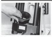
Pump reservoir must be properly vented before operation. Release the pusher clip and slide pusher back. NOTE: Periodically lubricate the die ring with Weatherhead T-400-G lubricant. When crimping with Coll-O-Crimp® I tooling, insert the T-420-25 adapter die ring into the base plate. Insert the proper sized collet.
