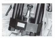
Loosen knob and tilt press as necessary. Insert hose assembly from below the base plate and between the collet halves. Align dimples or knurl band on end fitting with top of collet, making sure that collet halves are evenly matched.
