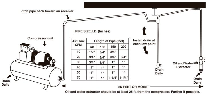
Adjust your air compressor air pressure to 90-120psi, (6.21-8.28 Bars). *NOTE:*
