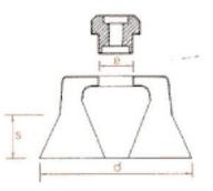
According to above drawing, 3.1/4" diameter, 1.1/8" trim length. Total N° of .020" wire ends in the brush: 2,160 Weight of total product: 500 gr.
