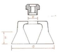
According to above drawing, 3.1/4" diameter, 1.1/8" trim length. No. of knots: 22 No. of .032" wires per knot: 28 Total N° of .020" wire ends in the brush: 1,120 Weight of total product: 610 gr.
