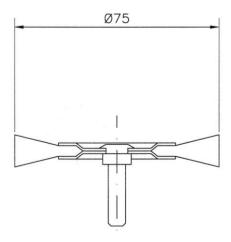
According to above drawing, 3" diameter, Total  $N^{o}$  of .012" wire ends in the brush: 4,000 Weight of total product: 75 grs.
