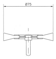
According to above drawing, 2.1/2" diameter, Total N° of .012" wire ends in the brush: 3,600 Weight of total product: 65 grs.
