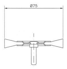
According to above drawing, 2" diameter, Total N° of .008" wire ends in the brush: 3,600 Weight of total product: 60 grs.
