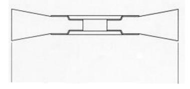
According to above drawing, 4" diameter, 11/16" trim length. 5/8" face width.
