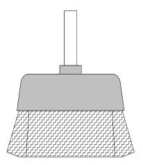
According to above drawing, 3" diameter, 3/4" trim length. Total N° of .012" wire ends in the brush: 2,400 Weight of total product: 120 gr.
