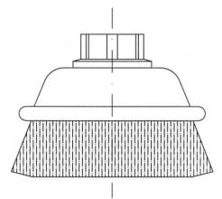
According to above drawing, 3" diameter, 7/8" trim length. Total  $N^{\circ}$  of . wire ends in the brush: 720x12 Weight of total product: 310 gr.
