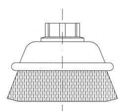
According to above drawing, 3" diameter, 7/8" trim length. Total N° of .012" wire ends in the brush: 4,800 Weight of total product: 310 gr.
